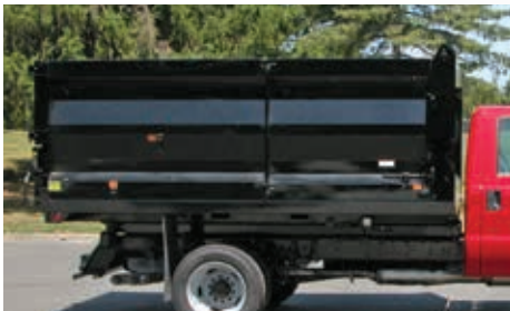
Durable 14 gauge steel front and side construction helps the Rugby Landscape Body stand up to the toughest working conditions.
