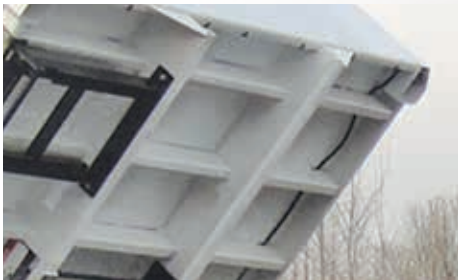
The Rugby Landscape Body's interlaced understructure provides added strength and rigidity.
